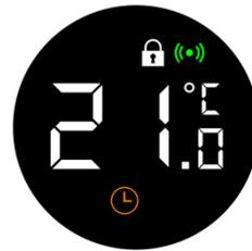
2. A symbol
